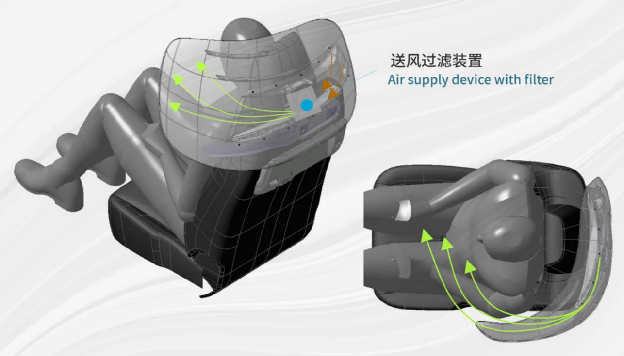
形成空气对流防护罩,隔离污浊空气 Air convection protective cover to shield dirty air
