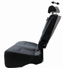
Rear seats Two-stage reclining mechanism (6 degrees of lean)
