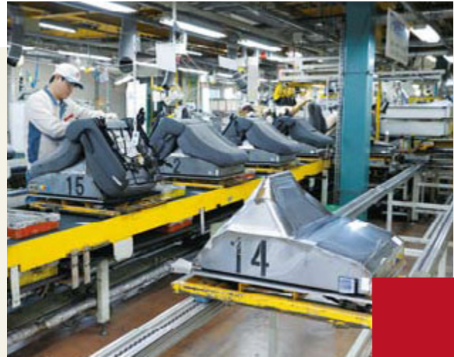
The protruding jig enables work to be easily performed on the backside of the chair portion of the seat.
