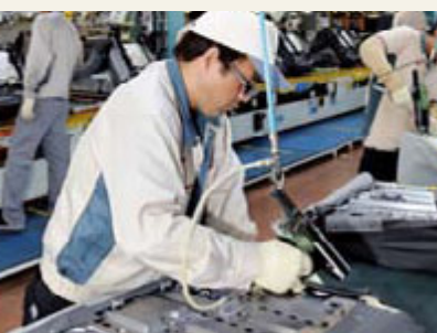
Work operations using hog ring pliers that can be freely moved 360 degrees
