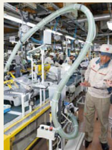
Only the needed clips are sent through a hose using air pressure.
