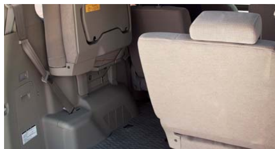
One-touch Folding Third-row Seat (used in Toyota Voxy & Noah) Stows away smoothly with a single touch.
