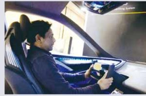
The cabin space model assumes Level 4 autonomous driving. The camera installed inside the vehicle and the sensor embedded in the seat implement four 'human-centred' systems including the maintenance of wakefulness, personal air-conditioning, automatic posture/ physical build detection and adjustment, and an emotion-linked interior.
