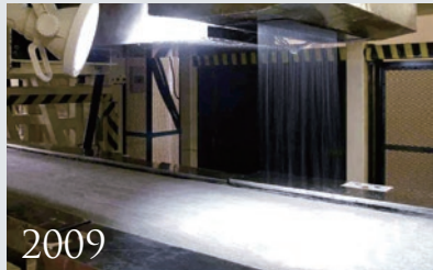
2009 Started production of cabin air filter material using the Dual Layer Melt Blown Method
