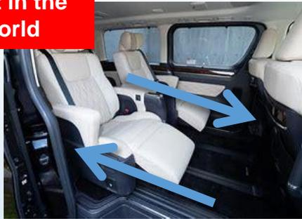
While adjusting the front slide, forward sliding by the seat's own weight can be inhibited.
