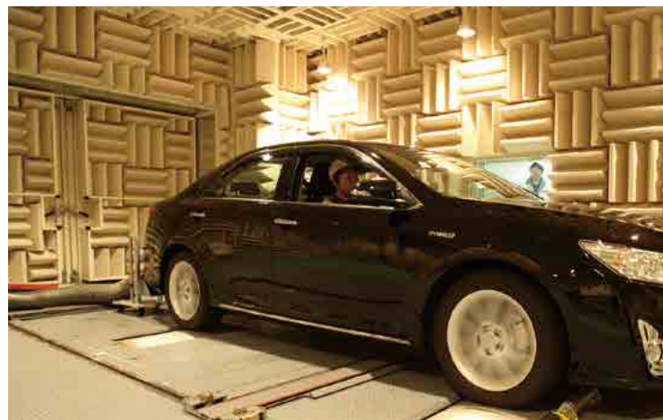
Analysing air intake noise by estimating noise when the engine is running and analysing frequency transmission characteristics
