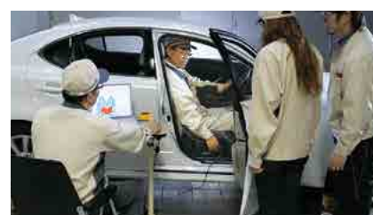
Seat pressure distribution analysis
