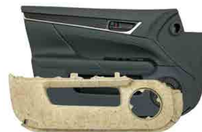
Door trim using kenaf base material
