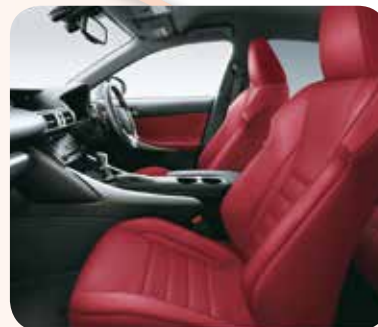
Seats utilising the Foam in Place Method
