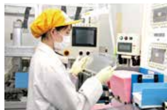
Inspection process for separators conducted under strict control for dust, temperature and other factors
