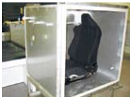
Measuring VOC levels using SUS box method
