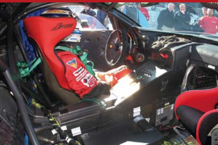
HANS seat built into the cockpit of the racing car
