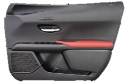
Door trims made with kenaf base material
