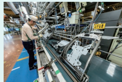
There was significant strain during work due to poor posture, so a device was introduced that reduces the burden by raising the frame.
