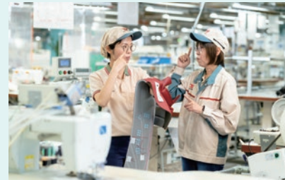
Pointing to the eye and raising the finger up to indicate stitch skipping (a defect whereby the yarn skips stitches)
