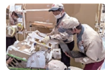
Simulation of the actual production process reproduced in cardboard
